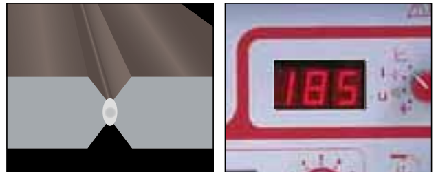
Penetration pass Short-Arc MIG, thickness < 25 mm.
