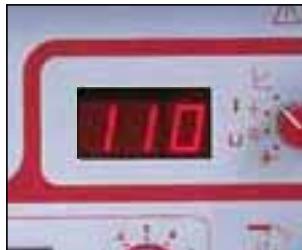
Short-Arc MIG, thickness < 3.0 mm.
